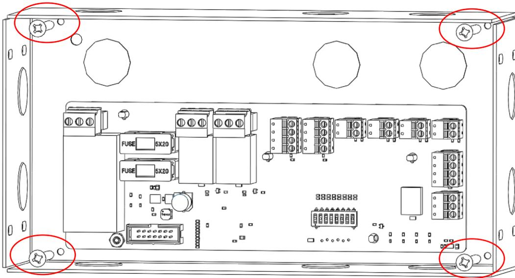
Figure 6: Surface Mount Installation
