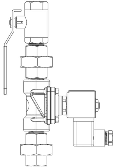
Figure 10: ISIMET Gas Valve Assembly
