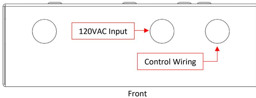
Figure 5: Example of typical wiring knockouts for the FLA (Top View)
