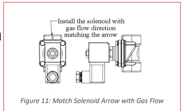
Figure 11: Match Solenoid Arrow with Gas Flow
