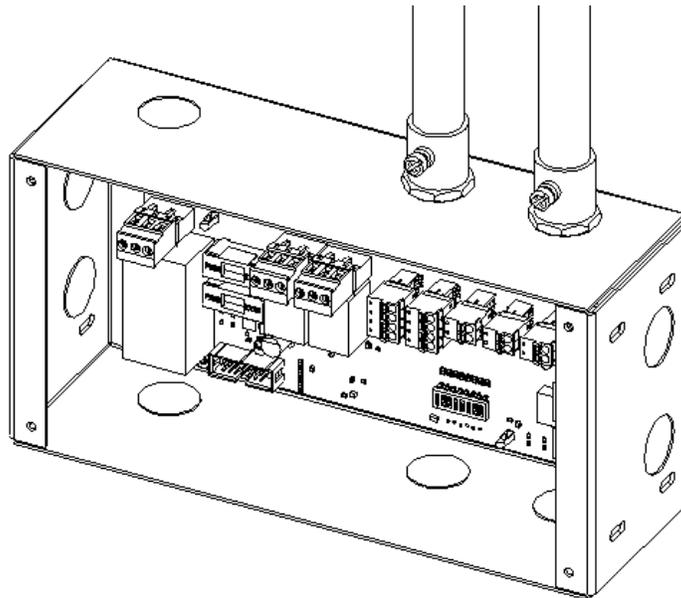
Figure 4: Recommended EMT conduit installation for FLAv2
