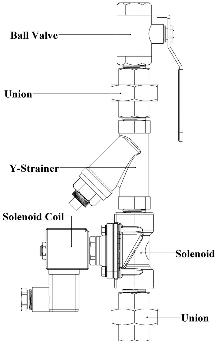
Figure 9: ISIMET Gas Valve Assembly with integrated Y-Strainer
