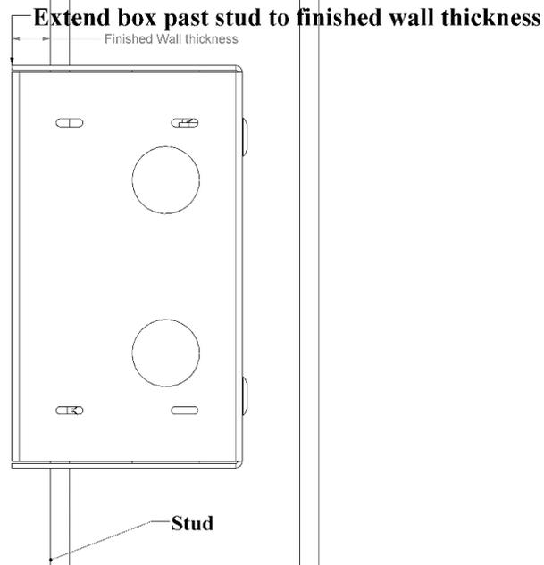
*Figure 1: Flush Mount Installation (Protrude to finished wall thickness)*
