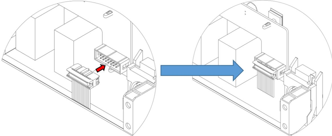
Figure 15: Attaching the Ribbon Cable from the FLA Daughterboard to the FLA Motherboard
