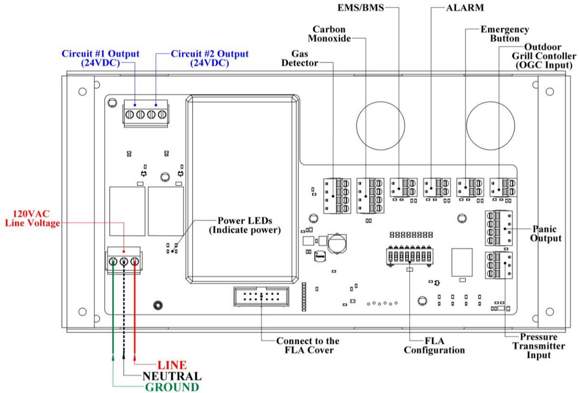
Figure 13: FLAv2 (Low-Voltage) Wiring Diagram
